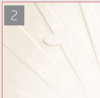
Turn the tray over, Note the raised circles in the base of the tray FIG 2, these are the feet location points and the feet must be fitted to these points and ONLY these points since they have been strategically placed to eradicate any flexing within the shower tray.
