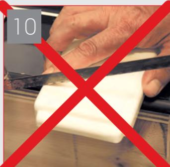
Please note on square and rectangle trays one length of panel has a return rebated end. Ensure that this end is included in the length required. Do not cut off and discard.
